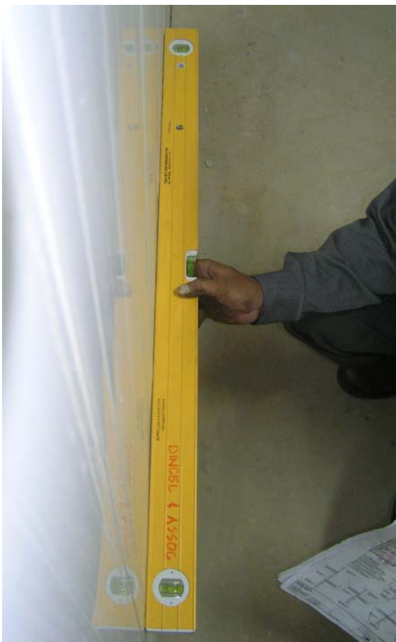
(200mm wall straightness several days after concrete fill)
